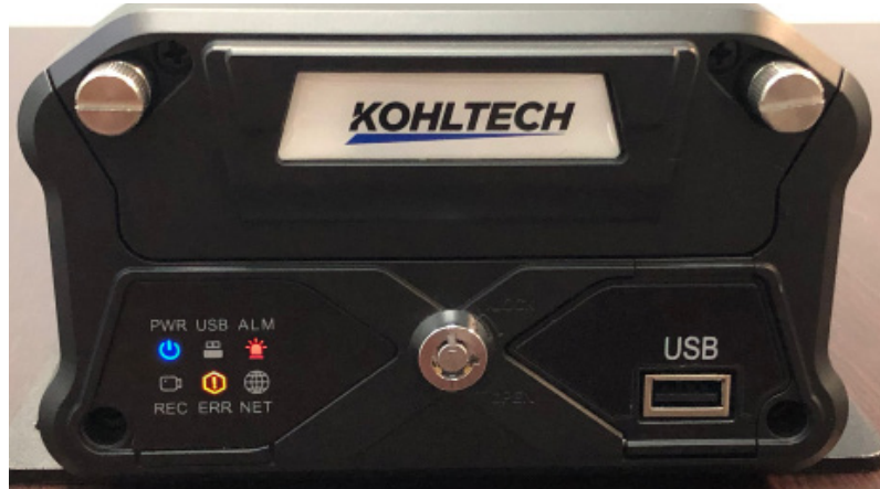
A orange ERR and red ALM light indicates a missing or damaged SD card and a disconnected or damaged camera.
