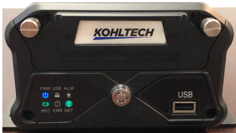
Normal operation with KOHLTECH Server connection - Blue PWR, Green REC and flashing Green NET light
