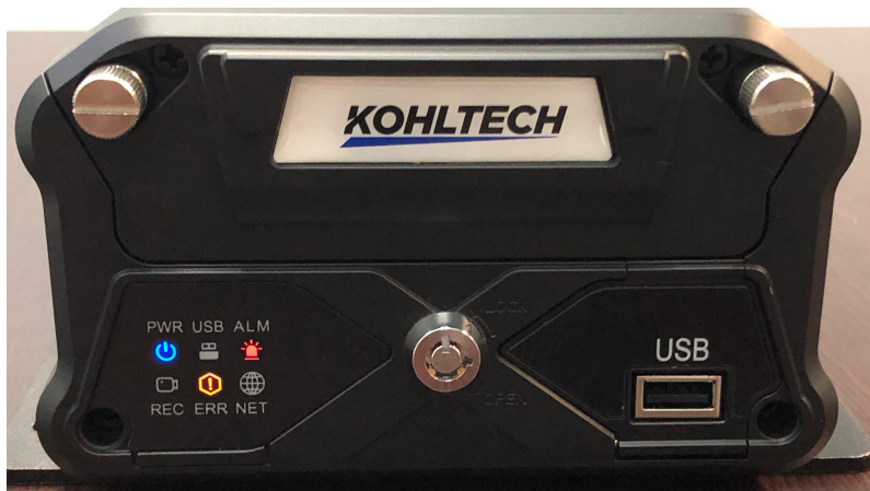
An orange ERR and red ALM light indicates a missing or damaged SD card and a disconnected or damaged camera.
